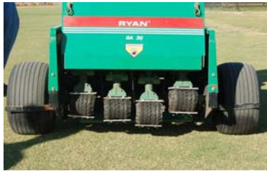
The Cady, originally built by Michigan State researchers using a Ryan GA-30 aerator and fitted with cleats, is used for traffic simulation on the Gainesville, FL NTEP bermuda
